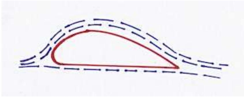
Required airfoil for light aircraft per Bernoulli's Principle
