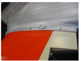
Here the wing has its finish paint while the fuselage and fairing are in aluminum paint. The fairing wraps around the leading edge and is a complex shape with several attachments to duplicate.
