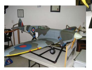
• Hangar 9 - 1/5<sup>th</sup> scale Spitfire Mk IXc 30cc. Airplane is outfitted with a DLE 35 RA. The plane has a nice top hatch with access to receiver, switches, throttle and choke servos.
