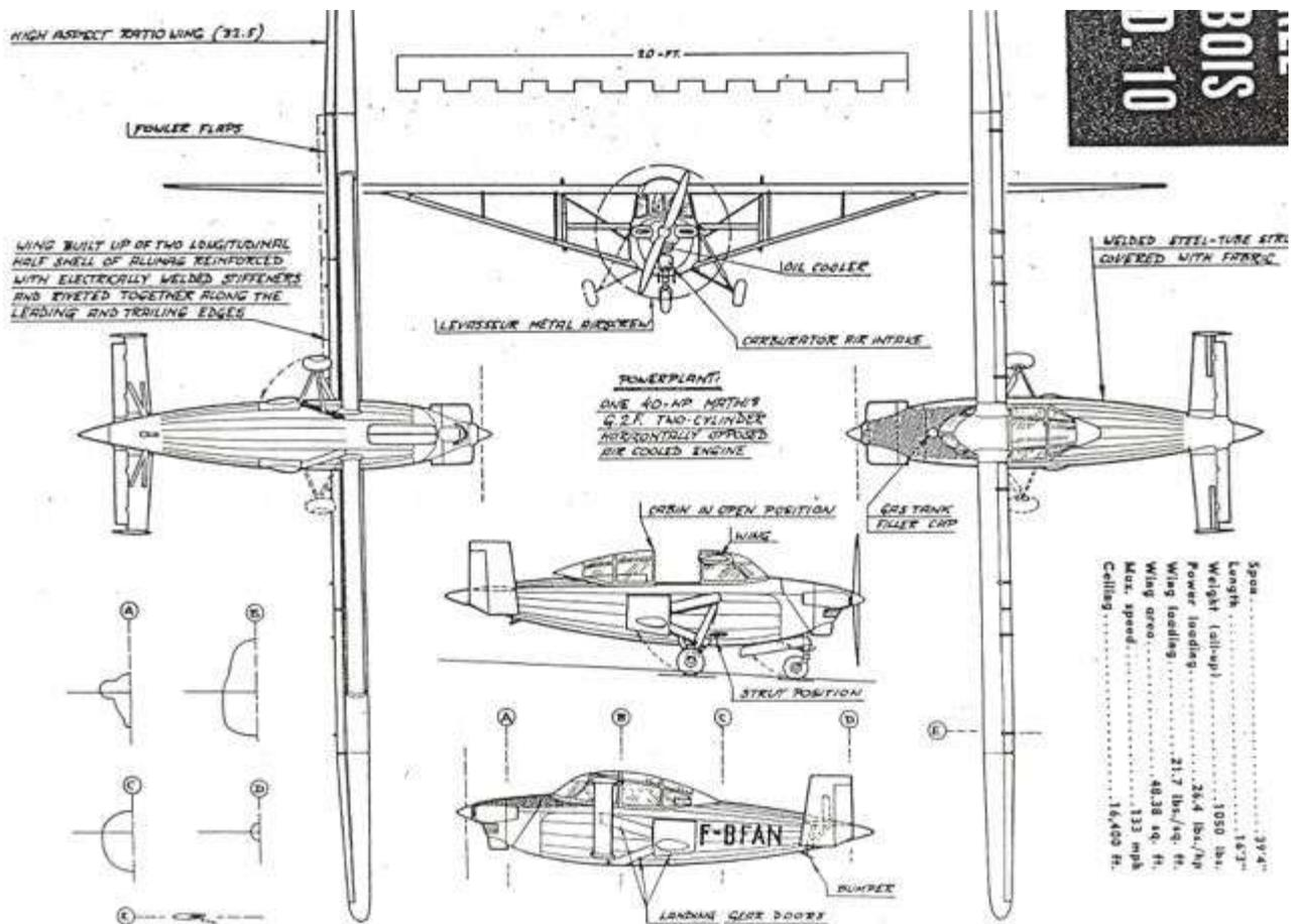
The HD-10 Proof of Concept aircraft was first flown in 1948. The performance of the unconventional Strut-Braced-Wing (SBW) or Truss-Braced-Wing (TBW) showed exceptional performance and very long range and resulted in a contract for two twin-engine cargo planes. The HD-31 first flew in 1953.
