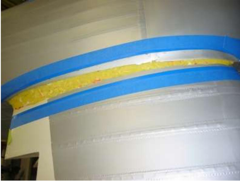
At this point you need to protect the models painted surface with a mould release. This can be a couple of layers of paste floor wax, or a coat of Poly Vinyl Alcohol. Also known as PVA it is a thin liquid that dries to a thin surface that is water soluble and nothing sticks to it. When the epoxy sets up you can just 'pop' the part off the surface.
